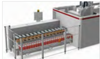
Linear tool changer with 50 positions
